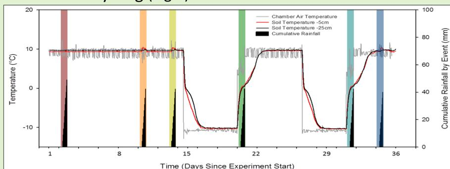
Fig. 2. Chamber air temperature, soil temperature, and rainfall events over the simulated non-growing season.
