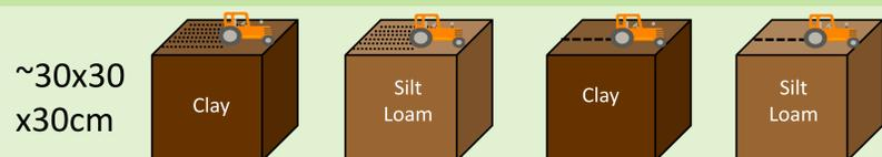
Fig. 1. Intact no-till clay and silt loam soil monoliths were fertilized via surface broadcast or subsurface placement in a laboratory.
