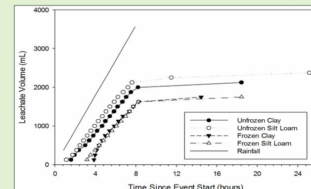
Fig. 4. Average timing of drainage of soil across unfrozen and frozen events, compared to rainfall inputs.
